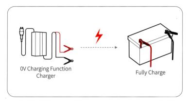
The charger can charge the battery starting from OV.
