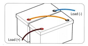
After series connection, the voltage of the battery system will be doubled according to the number of batteries you connect. E.g. If two 25.6V150Ah batteries are connected in series, the battery system will be 48V (51.2V)150Ah
