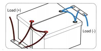
After parallel connection, the capacity of the battery system will be doubled according to the number of batteries you connect. E.g. If tw 24V150Ah batteries are connected in parallel, the battery system will be 24(25.6V)300Ah
